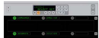
Cabinet is shown with LOCALE display. Adjacent to Language is the current language choice; adjacent to Degrees is the current temperature range.
