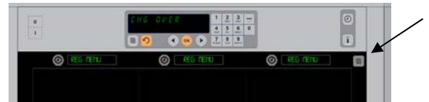
Pressing the row mode button (see arrow) produces a sequence of menu choices. With the desired menu for the row displayed, press the OK button on the top keypad.
