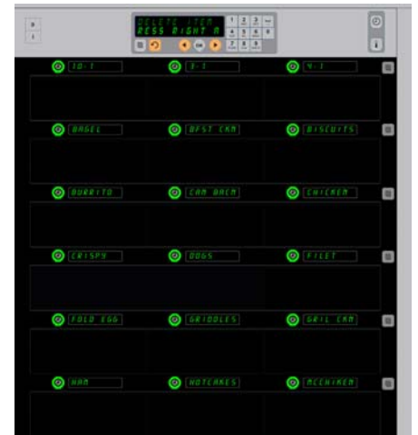
Cabinet with menu items displayed. The item to be deleted is chosen with a timer key. The deletion is confirmed with the OK key on the controller.
